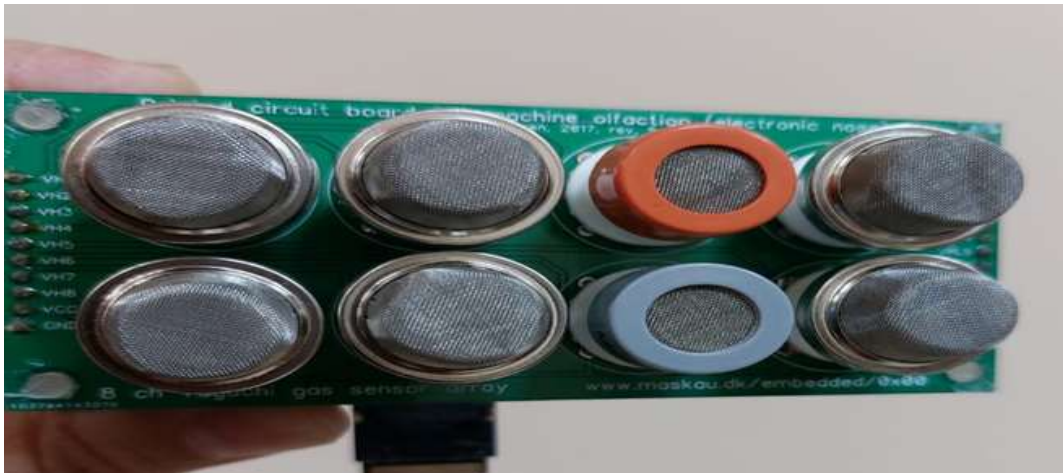
Figure 8: A prototype electronic nose (EN) with eight metal-oxide semiconductors (MOS) sensors.
