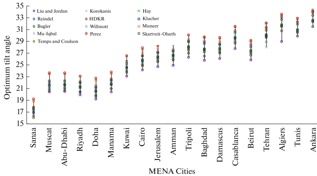
Fig. 1. Optimum tilt angles of solar collectors for MENA cities according to all transposition models.
