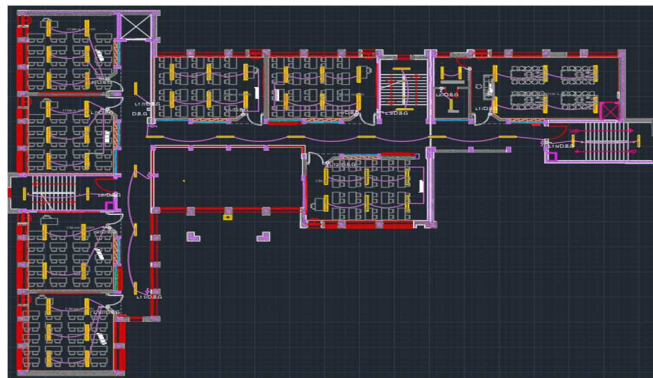
Fig. 2. Lighting distribution for the first floor.
