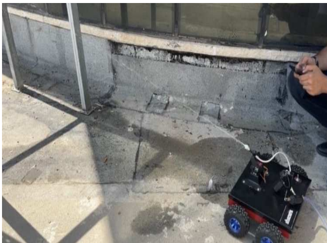
Fig. 7. Testing direction of robot motion, direction of the water pump arm and pumping tasks.
