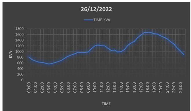
Fig. 1. Load curve for all transformers in 26/12.
