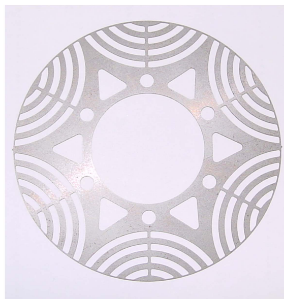
Figure 6. Cross section of the synchronous reluctance machine.
