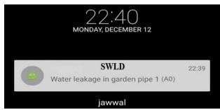
Figure 27. Result when leakage detected in region 1
