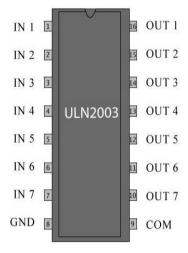
Figure 12. ULN2003 structure and pins classifications
