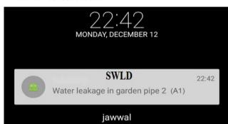
Figure 28. Result when leakage detected in region 2
