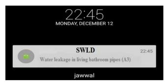
Figure 30. Result when leakage detected in region 4
