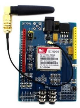
Figure 7. SIM900 for Arduino controller
