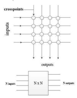
Figure 1: *N* x *N* Crossbar switch concept.
