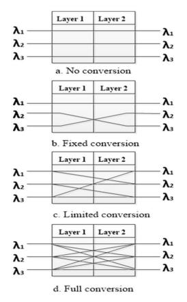
Figure 3: Wavelength conversion types.
