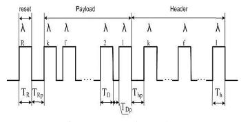
Figure 7: Format of the packet.
