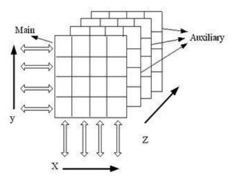
Figure 5: Multi-layered architecture of switching matrix.
