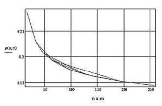
Figure 8: Dependence of switchboard load factor on the sizes of the switchboard  $m \times n$ .
