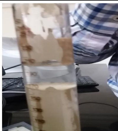
Figure 5.2: The growth of SRB in the enrichment media in the column after 6 weeks.
