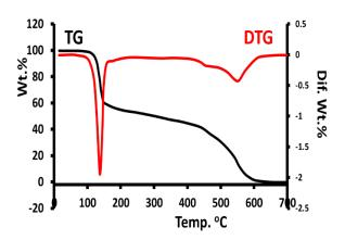
Figure (1): TG/DTG thermal curve of SB
