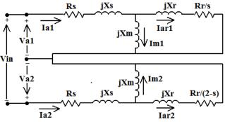
Figure (3): The sequence network equivalent circuit.
