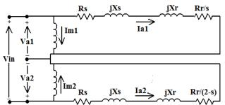
Figure (4): A simplified approximate sequence network equivalent circuit.
