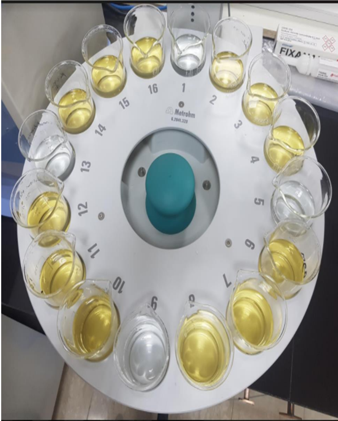
Figure 7: The auto-sampler 16 positions with 12 tested samples and 4 water samples for cleaning the sensors.
