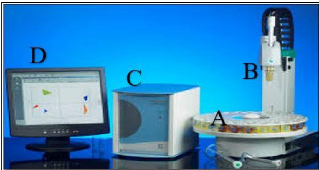
Fig. 6. Alpha MOS Astree II ET parts: (A) liquid autosampler, (B) electrochemical sensor array, (C) acquisition unit, (D) Alpha Soft software (Alpha MOS, 2009).
